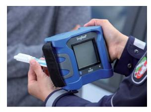
The DrugRead hand held device provides user-friendly interpretation of DrugWipe S saliva tests. Perfect for use at roadside checkpoints or police stations, the DrugRead offers precise time keeping, analyzes and documents the results of DrugWipe S drug tests for later use.
